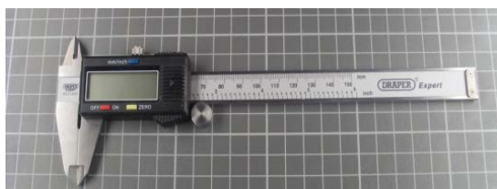
(Figure 1) Electronic Mitutoyo callipers used for manual measurement
